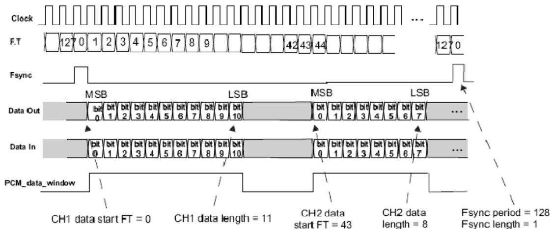
**FIGURE 3:** Two channel bus timing
