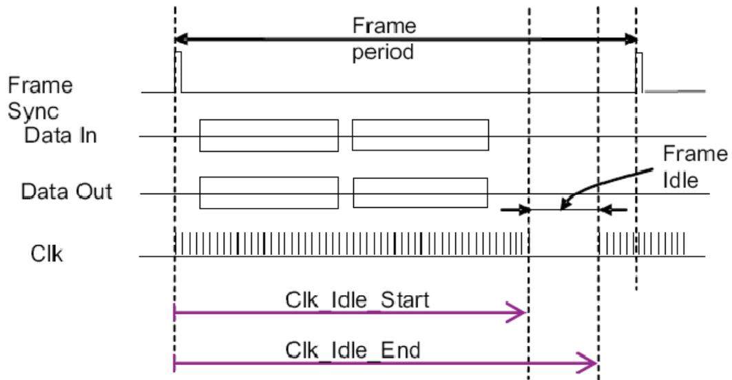
**FIGURE 1:** Frame timing description.
