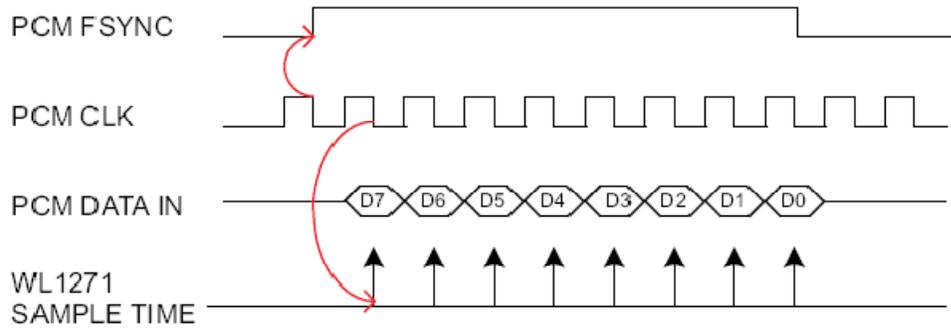
**FIGURE 2:** Negative Clock PCM Operation.
