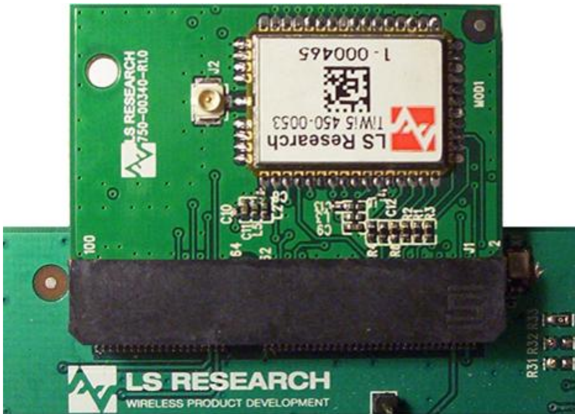
Figure 4 COM6L-T5 Attached to Host PCB with Mating Connector
