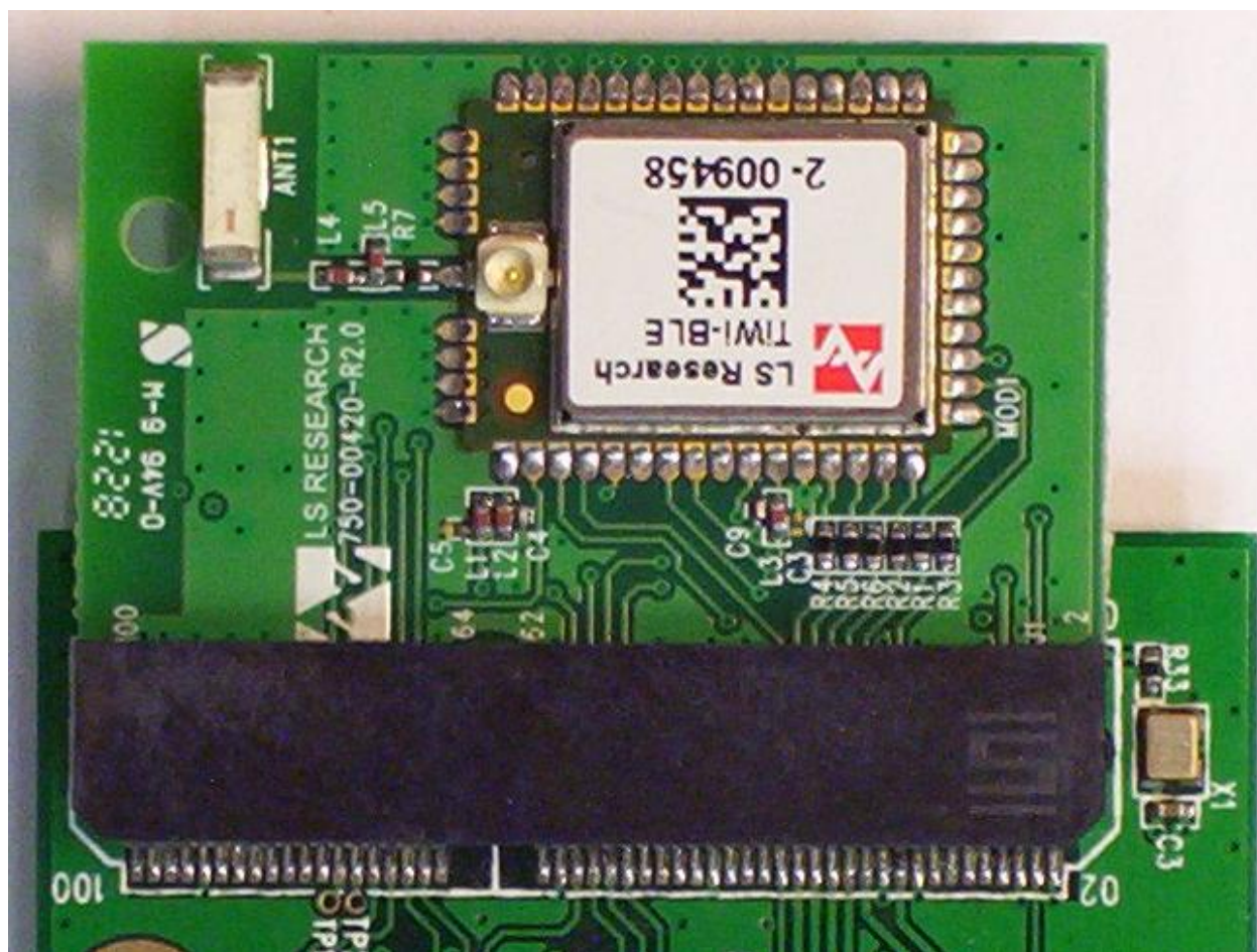
Figure 6 COM6L-BLE Attached to Host PCB with Mating Connector
